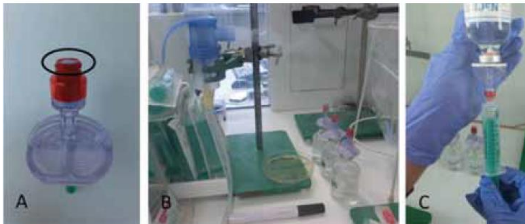
(A) Safeflow valve integrated in Mini-Spike® 2 Chemo; (B) Experimental setup; (C) Withdrawal of NaCl after nebulisation
